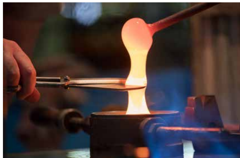
Coupe de cristal en fusion / Cutting during the hot glass process
