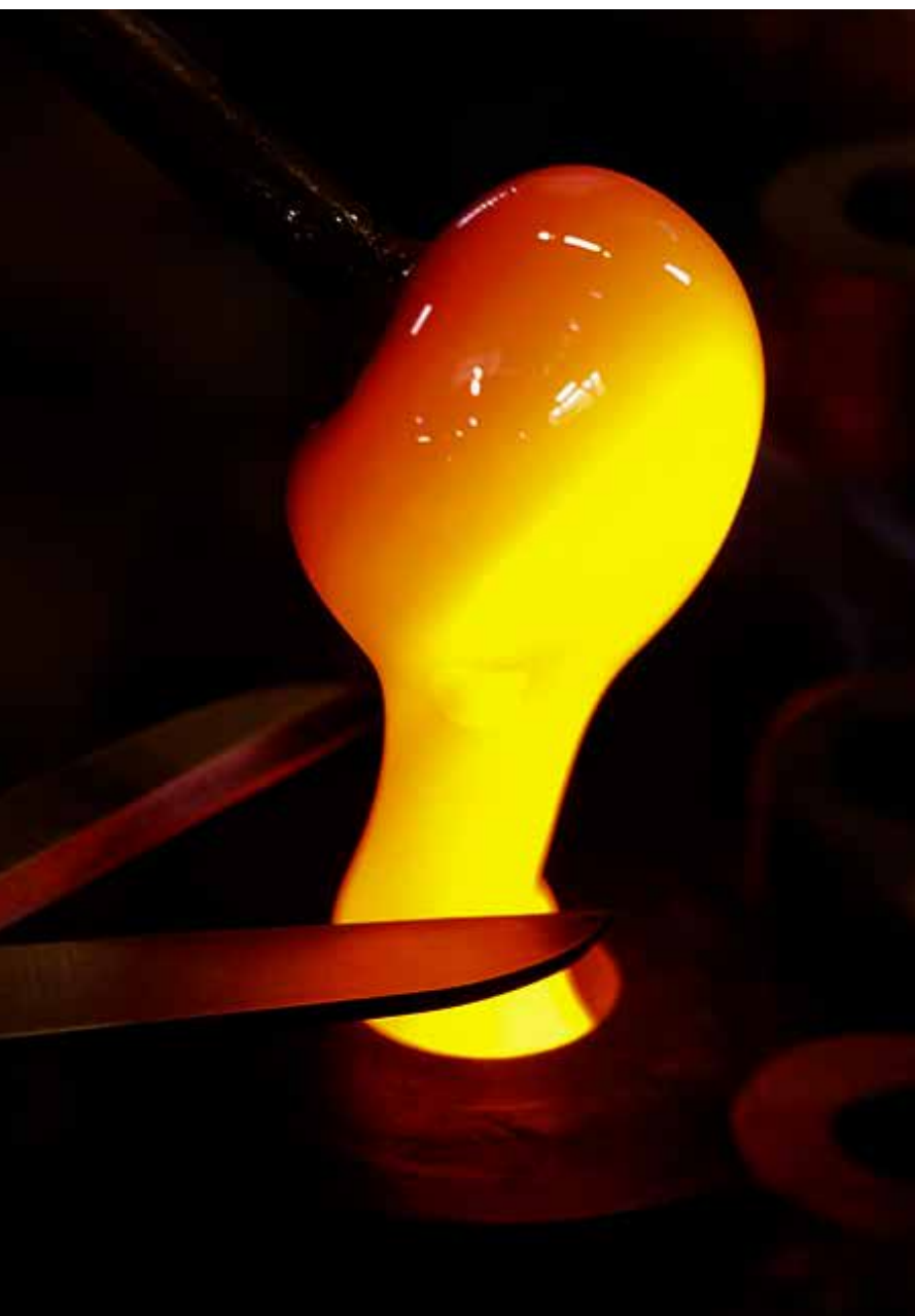
Coupe de cristal en fusion / Cutting during the hot glass process
